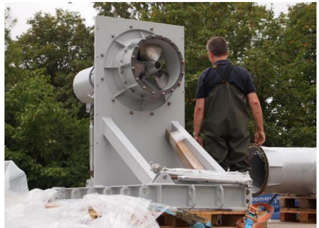
Visual 2: Axial Propeller turbine of VETT system in Eaton Socon.
